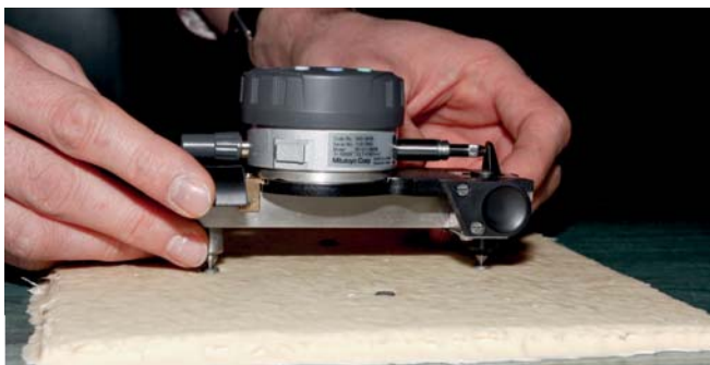
Fig. 5. Extensometer used for length change measurement
