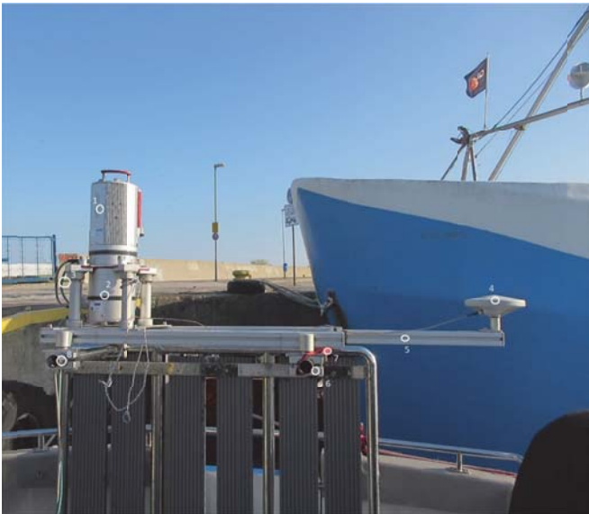
Fig. 3 Components of the Riegl VMZ-400 system on a vessel 1. Riegl VZ-400 laser scanner. 2. IMU. Connection cables between the scanner, 4. IMU, power source and laptop.5. GNSS antenna.6. Aluminum frame on which individual components are mounted.7. Aluminum clamps securing the platform to the elements of the vessel.8. Straps that fasten the platform to better stabilize the entire platform
