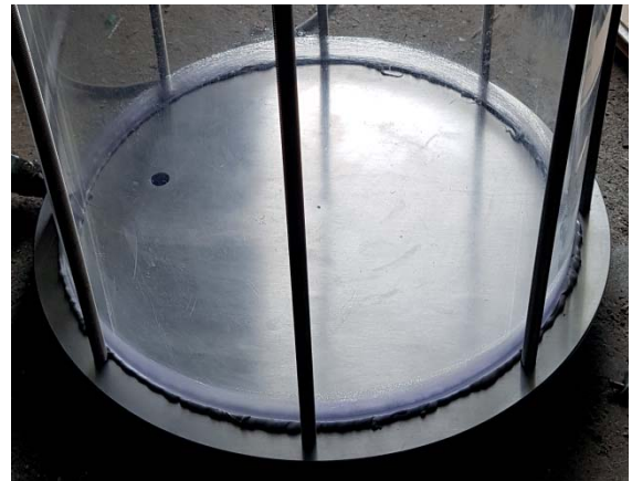
Fig. 8. Sealing of lower tank
