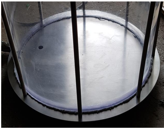
Fig. 8. Sealing of lower tank
