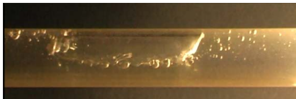
Fig. 3. Small bubble formed in the slug flow.
