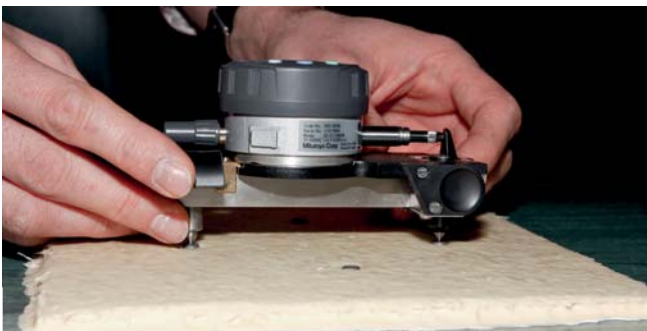
Fig. 5. Extensometer used for length change measurement
