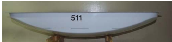
Fig. 5 Side view of the model without appendages
