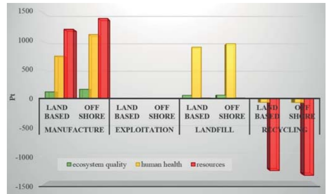
Fig. 9. Results of grouping and weighting of environmental after-effects for three areas of impact, in consecutive stages of material existence cycle of wind power plant blades, taking into account possibility of their post-consumer reuse [own research]
