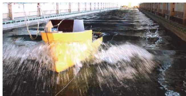
Fig. 1. The seakeeping tests in the CTO S.A. deepwater towing tank.
