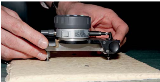
Fig. 5. Extensometer used for length change measurement
