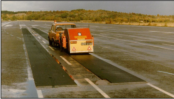
Figure 1. Tire/road noise measurements on PERS section located on Torslanda Airport.
