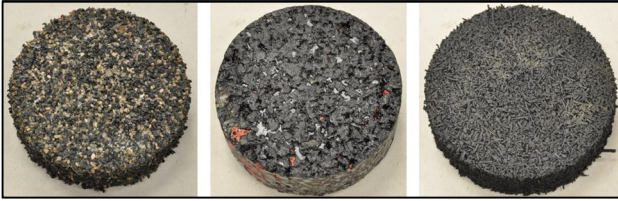
Figure 4. Selected samples used for stiffness evaluation; from the left: PERS - A, low noise asphalt pavement COLSOFT, PERS - B
