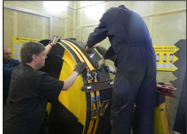
Figure 3. Bonding PERS ribbon to the drum
