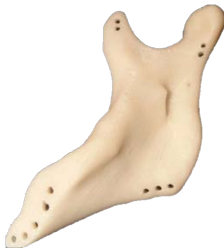
Fig. 5. 3D printed mandible implant prototype
