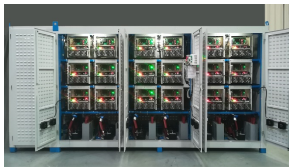
Fig. 2. Air-cooled 4kV/4kV PET, constructed from 1.2kV SiC MOSFET power modules (Photo courtesy of MMB Drives )
