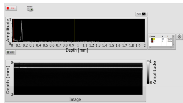
Fig. 4. Single A-scan (above) and OCT image (below) of polyurethane belt. Normalized amplitude corresponds with pixel brightness on the image and the frequency scale (obtained in FFT) can be used to map data to depth profiles.
