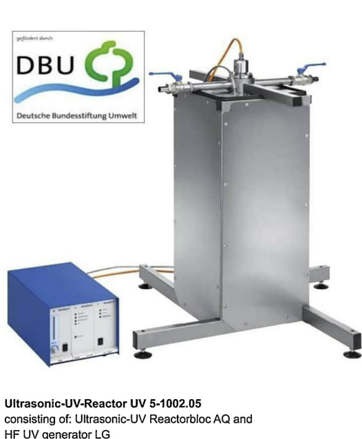
Fig. 1. Experimental setup for acoustic cavitation.
