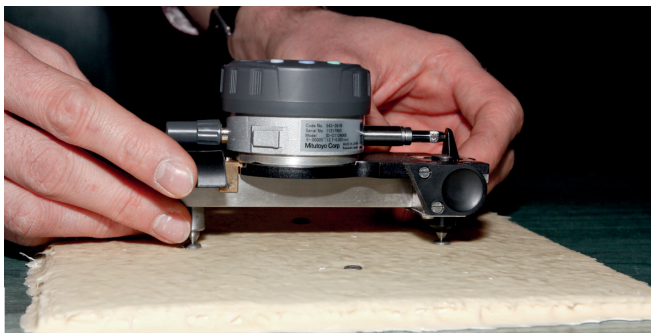
Fig. 5. Extensometer used for length change measurement
