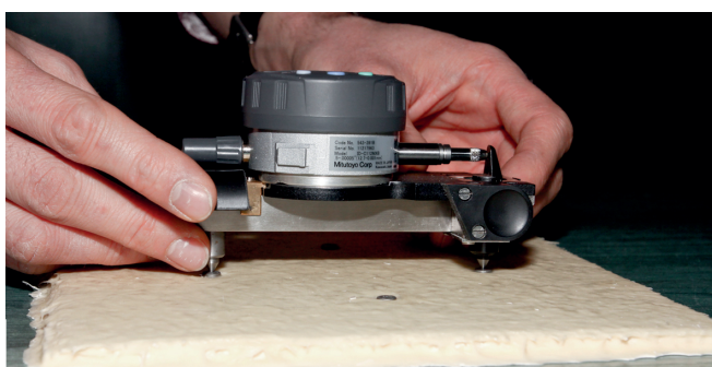
Fig. 5. Extensometer used for length change measurement
