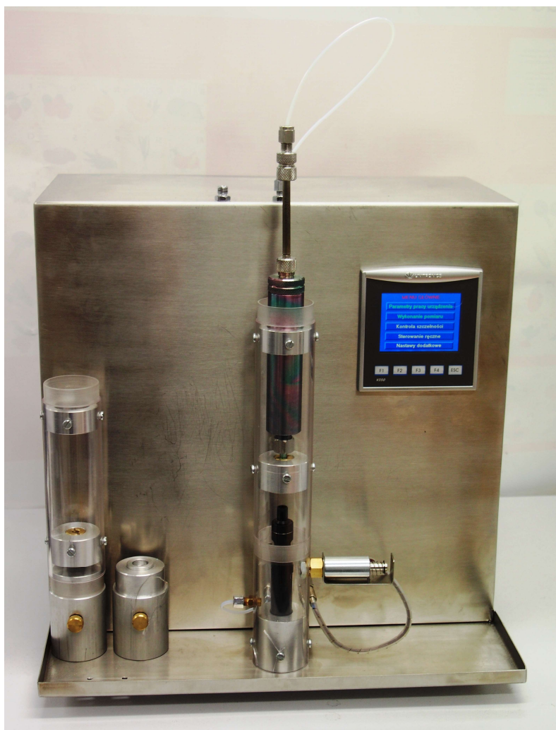
Figure 1. Automatic generator of aerosol from electronic cigarettes designed and constructed in the Department of Analytical Chemistry, Faculty of Chemistry, Gdańsk University of Technology
