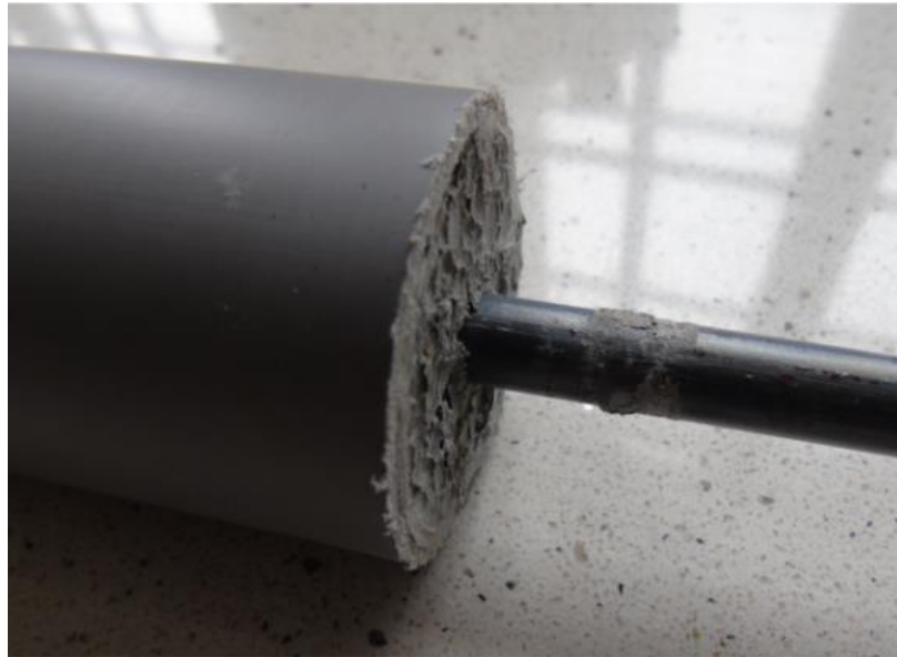
Figure 5.22. Failure mode of the anchor after pull-out procedure
