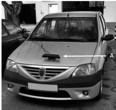
Fig. 5. A car equipped with a Kinect sensor (A).
