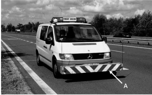
Fig. 1. A professional laser profilograph (A) mounted on a vehicle [11].
