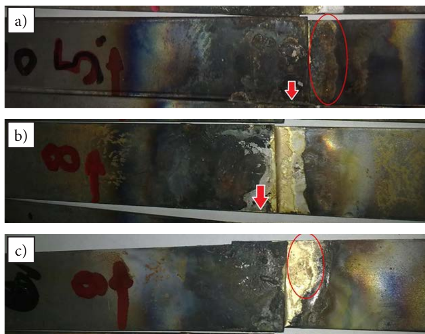
Fig. 2. Visual test results; a) specimen 5 – three copper inclusions, excessive spread of the brazing metal (ellipse), a crack of the braze and gas pores (arrow), the overlap on the upper edge not filled with the filler metal, b) specimen 8 – immersed in water, a crack of the braze (arrow), the overlap on the left edge not filled with the filler metal c) specimen 9 – provided with the flux used in the SAW method, excessive spread of the brazing metal (ellipse), gas pores, the overlap on the upper edge not filled with the filler metal
