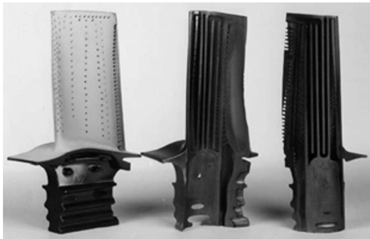
Figure 11: Gas turbine blades with cooling holes (left).
