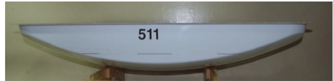
Fig. 5 Side view of the model without appendages
