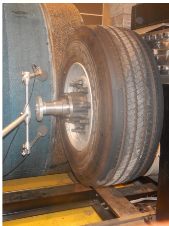
Figure 16: Truck tire/road noise testing on roadwheel facility at TUG
