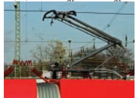
3. The current collector from the traction network (pic. Mario Schürholz www.bahnbilder.de)
