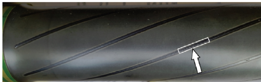
(c) Place of sample cutout for testing-depicted by arrow the sample size 0.526 mm×2 mm×14.64 m
