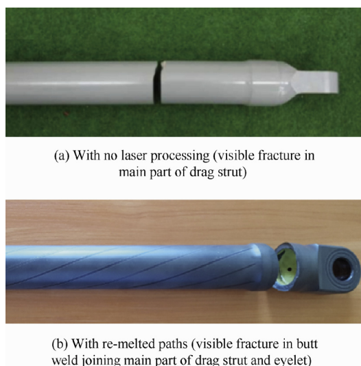
Fig. 7 Two drag struts of landing gear after testing fatigue.
