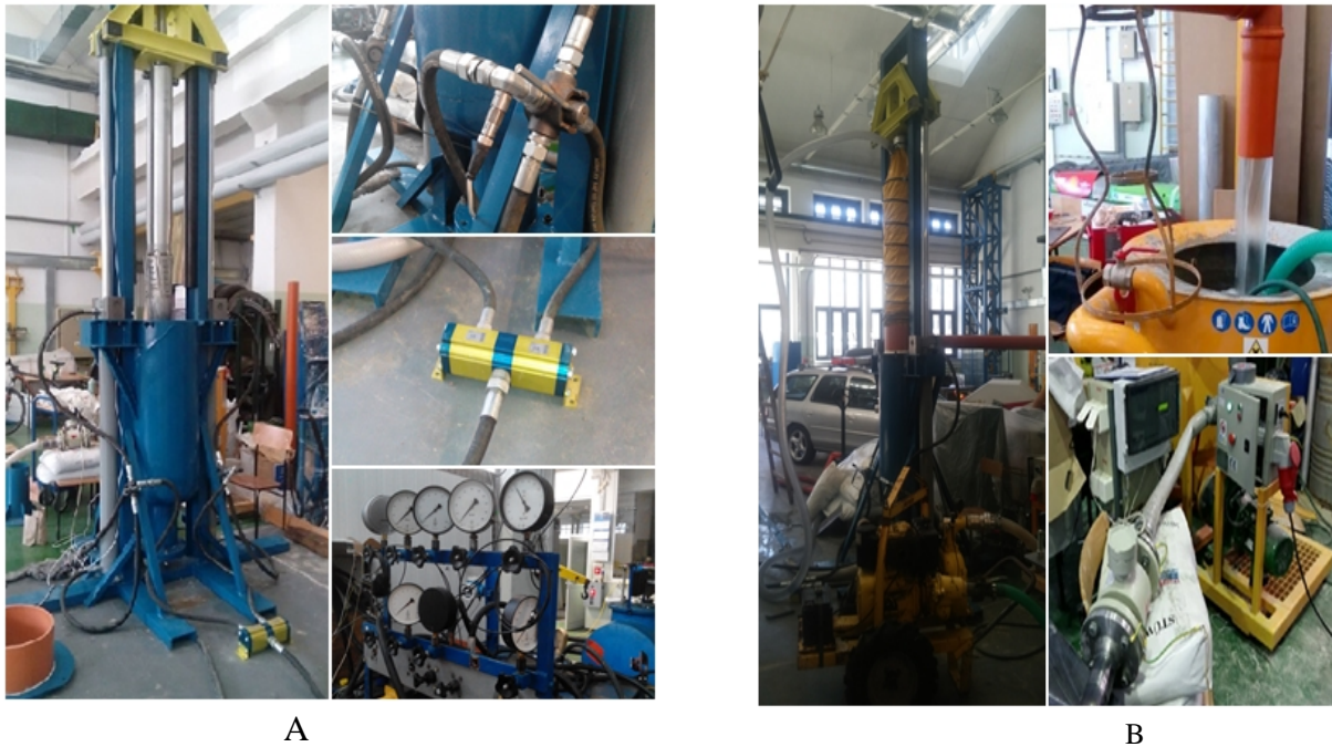
Fig. 7. Clay-cutting laboratory testing station at Gdansk University of Tehcnology: A – hydraulic system, B – mud circulation system.
