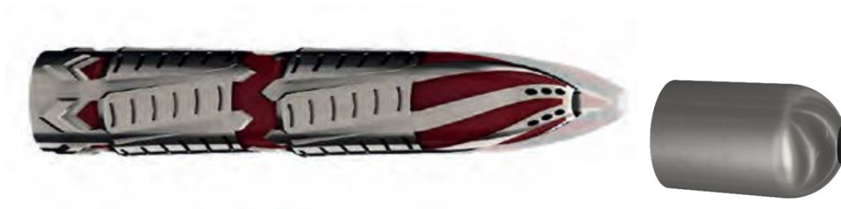
Fig. 8. Protector tool geometry and standard cementing shoe
