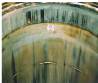
Fig. 4. Image of the damaged surface of cylinder liner due to an excessive friction wear resulting from the seizing of piston in the cylinder [30]
