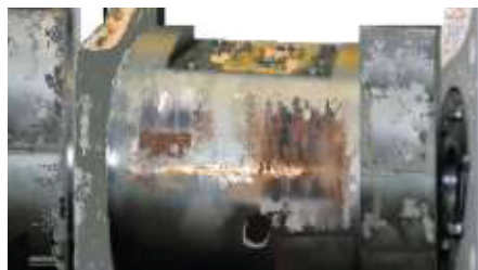
Fig. 5. Image of the damaged surface of crosshead pin resulting from an excessive wear due to friction and corrosion [30]
