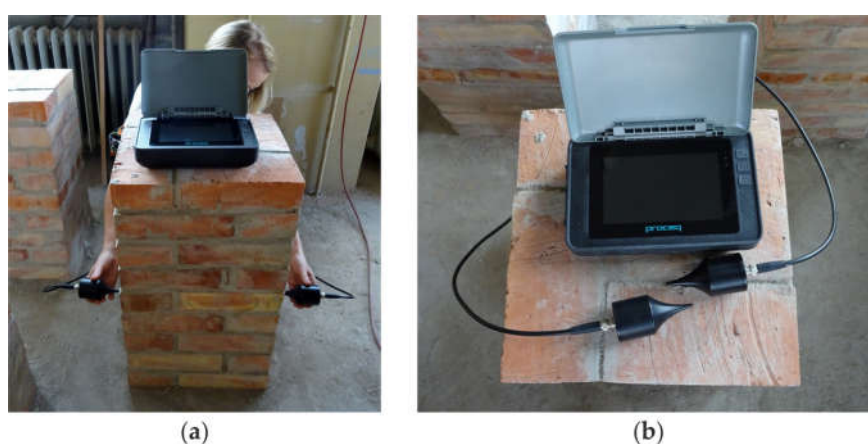
Figure 4. Experimental setup: (a) testing in through transmission mode; (b) registration unit and exponential transducers.
