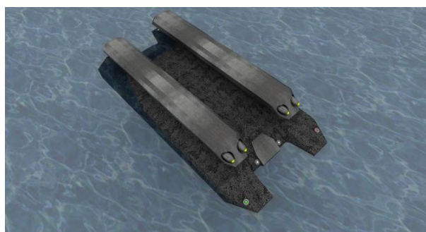
Figure 1. The general visualizations of the hull form and arrangement of external spaces of the stealth AUV vehicle (Gerigk, 2014-2018).
