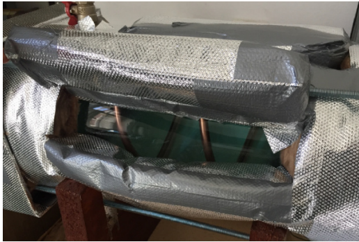
Fig. 3. View of the tested LHTE system
