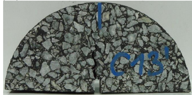
Fig. 3. Stone matrix asphalt SMA 8
