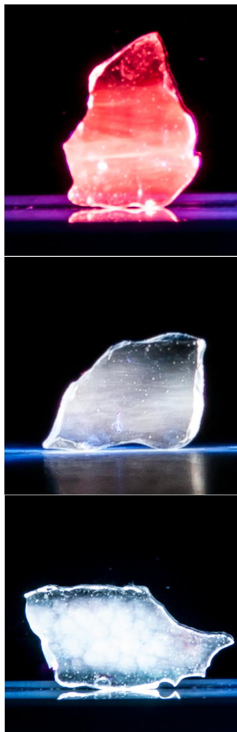
Figure 6: Photographs of photoluminescence of samples A (top), B (middle) and C (bottom) excited by a blue laser diode. The samples are ca. 1 cm high.
