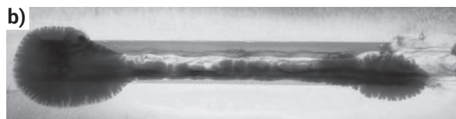
Fig. 4. Results of non-destructive testing for specimen W1, welded in the water, a) VT – wrong shape, b) PT – indication through the all length of the weld
