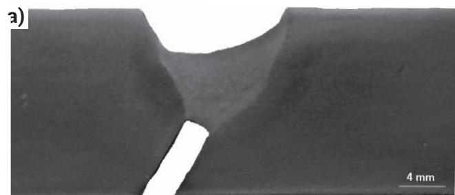
Fig. 7. Results of macroscopic testing for specimen welded in the air; a) Specimen P2.1, b) Specimen P2.2 – no imperfections
