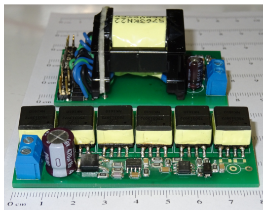
Fig. 13. MOFC vis-à-vis MTFC for the 6 isolated symmetric supply tracks \pm 15 V; (prototype setup height [mm]: MOFC-26; MTFC-12,5)
