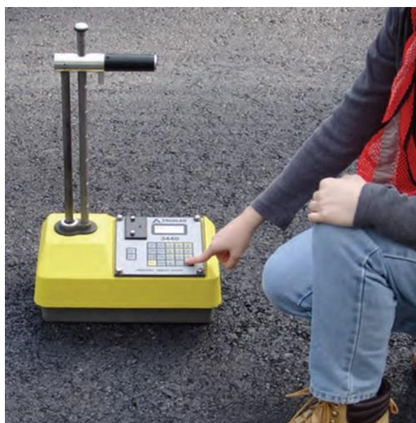
Rysunek 3.5 aparat NDG (VI Survey Instruments, 2014)
