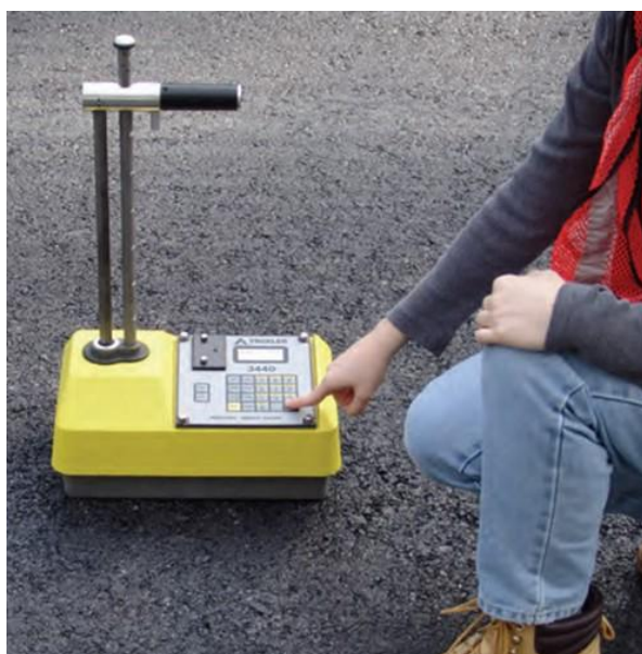
Rysunek 3.5 aparat NDG (VI Survey Instruments, 2014)
