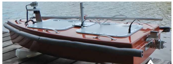
Fig. 12. UPP-1E universal measuring floating platform
