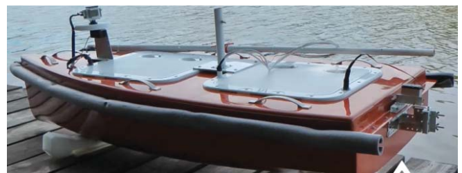
Fig. 12. UPP-1E universal measuring floating platform
