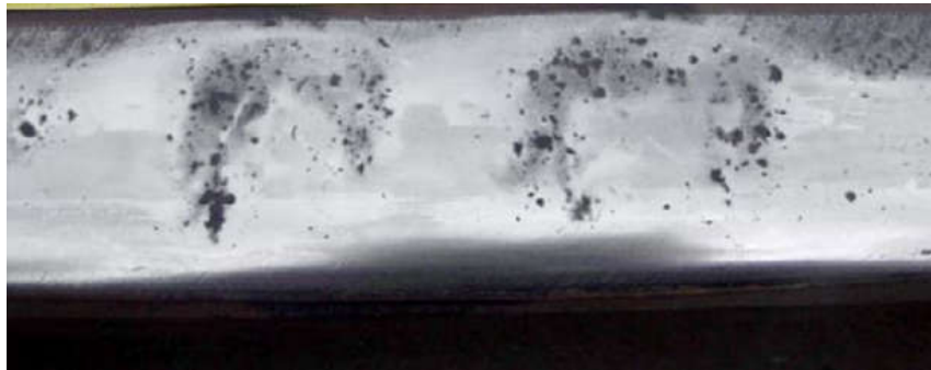
Fig. 2. Typical forms of squat-type defects: V-shaped crack (left) and arc-shaped crack (right).
