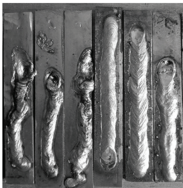
FIGURE 3. Exemplary specimens after pad welding, first three – welded in the water, second three – welded in air
