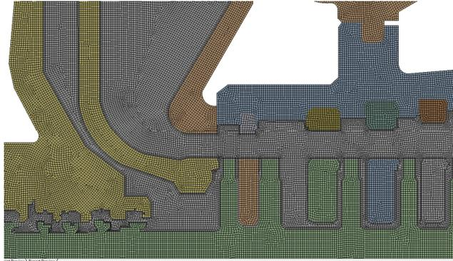
**FIGURE 4.** Discretisation of the fluid and solid domain.
