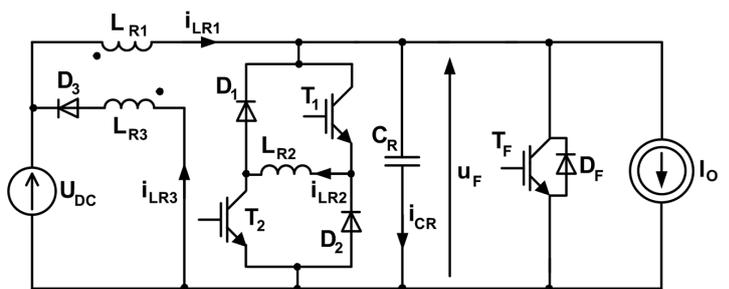
Fig. 7. Modification of the PCQRDCLI Link Inverter [12]
