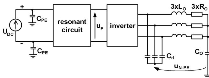
Fig.13. Simulation circuit for  $u_{N-PE}$  and  $u_F$  waveforms
