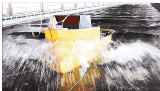
Fig. 9. The example seakeeping tests in CTO S.A.
