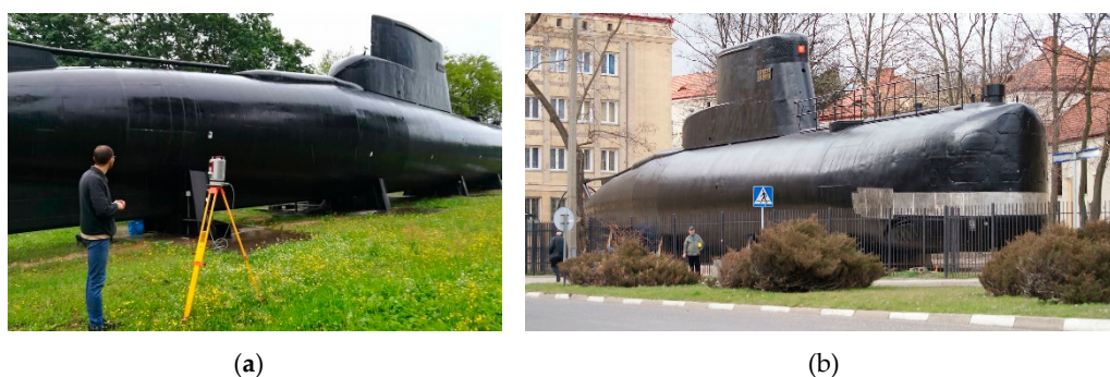
Figure 1. PNS Jastrzab—decommissioned submarine—object of research: (a) wet object during laser scanning with control points, (b) general view of the submarine (source: by Pawel Kusiak, CC BY-SA 4.0, https://commons.wikimedia.org/w/index.php?curid=42676502 ).
