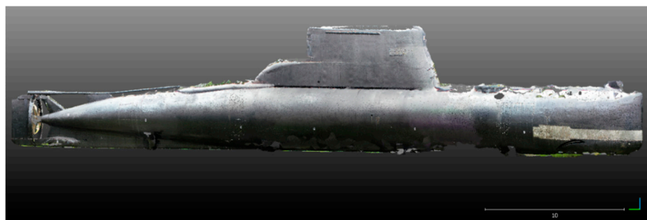
Figure 8. The object modelled with a photogrammetry technique (colored point cloud).
