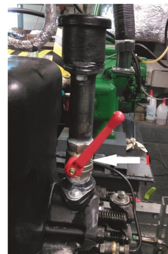
Fig. 1. A view of the inlet air duct supplying the engine: 1 – supply air control valve (degree of shutdown of the valve as during the laboratory
