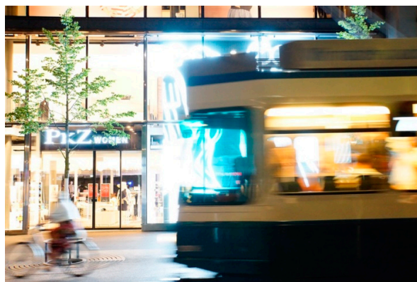
Figure 11. The “Walk” LED light art installation integrated into the facade of the PKZ Woman store on Bahnhofstrasse in Zurich, Switzerland. This was the largest of all the measured LED animated facade displays, and the disability glare it produces has a definite impact on traffic, negatively affecting tram drivers. Source: Julia Hartmann's figure.
