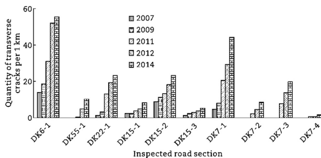
Fig. 9 – Quantity of transverse cracks at the observed road sections.
