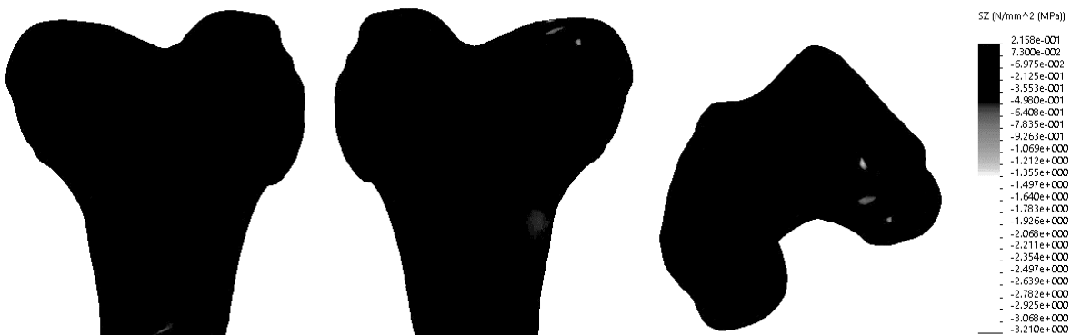
Fig. 11. Normal stresses along the Z axis (mechanical knee axis) of the proximal tibia (both materials – bone)
