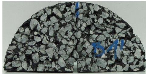
FIGURE 2. Stone matrix asphalt PA 8.
