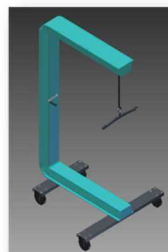
FIG. 1. 3D Model of the proposed patient transfer assist device.
