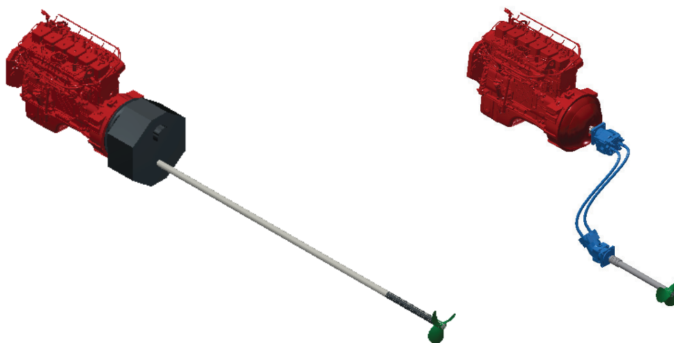
Fig. 1. Visualisation of inland vessel propulsion system (own elaboration) a) System with shaft line and mechanical gear b) System with hydrostatic gear
