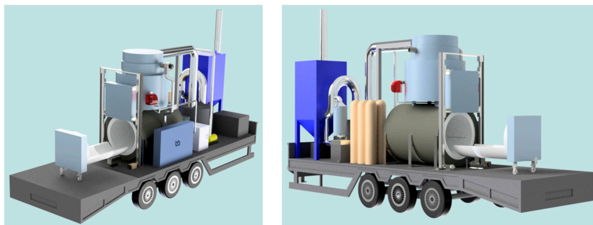
Figure 5. Visualization of the mobile medical waste incinerator.
