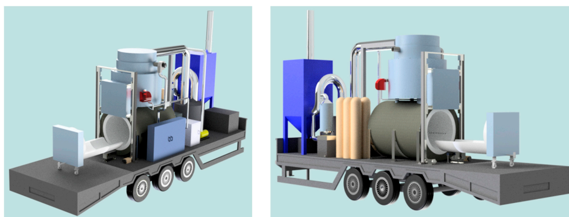
Figure 5. Visualization of the mobile medical waste incinerator.
