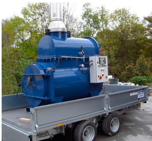
Figure 2. A view of the Matthews Environmental Solutions mobile incinerator [19].
