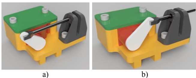
Fig. 5 Releasing mechanism, servo part a) open b) closed
