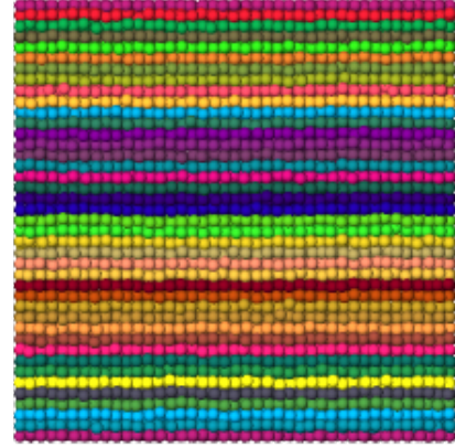
Fig. 4. Visualization of atoms grouped into subsequent crystal planes along Oz axis in OVITO [25]
