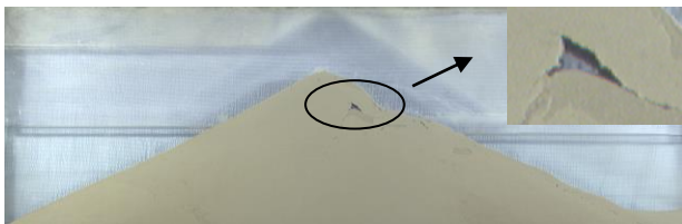
Fig. 3. Shape of the macropore at the end of the experiment, t=2000s .
