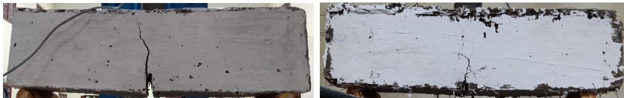
Fig. 13 Failure patterns for beams M0 and M4
