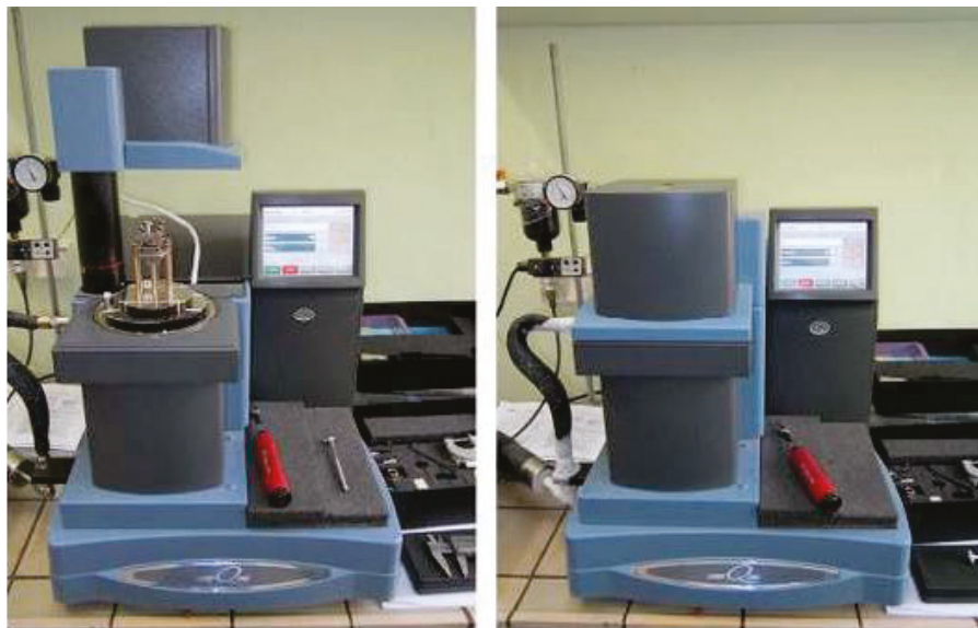
Figure 5. Test setup with dynamic mechanical analysis (DMA) Q800 analyzer.
